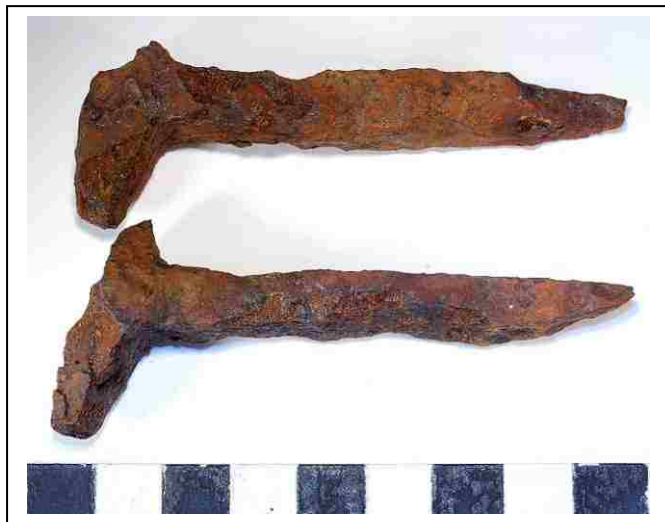
Fig. 6 Hand-forged nails with square shanks # DWA209IR/F10//MO5.
